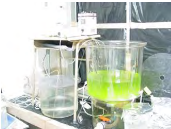
20 L-scale copepod culture system with continuous feeding system
